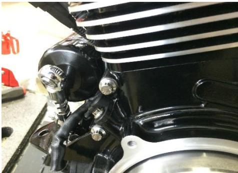
ARP cylinder studs hold the top end down while the rest of the drivetrain was fitted with stainless ARP 12 point fasteners. On the top side, heavy duty Delkron billet rocker shaft supports and S&S roller rockers were installed to handle the extra HP.
