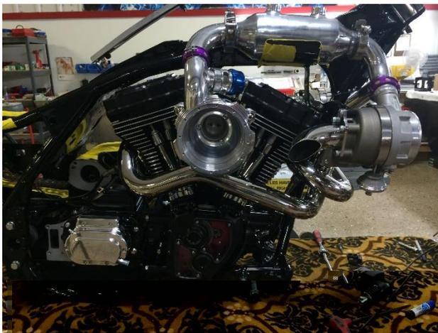
**Turbo system:** The turbo system we designed for this bike was quite a mechanical feat in itself. We're running two 53mm self-oiling Aerochargers, a custom made set of 304 stainless steel exhaust runners, an adjustable turbo smart Blow off valve along with combining both an Air/Air and optional
